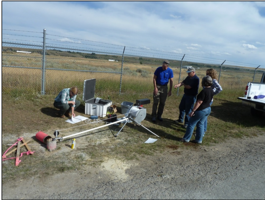
MTAML and OSMRE staff using OSMRE's bore-hole camera in one of the recently drilled holes (OSMRE site-visit, August 27, 2014)
